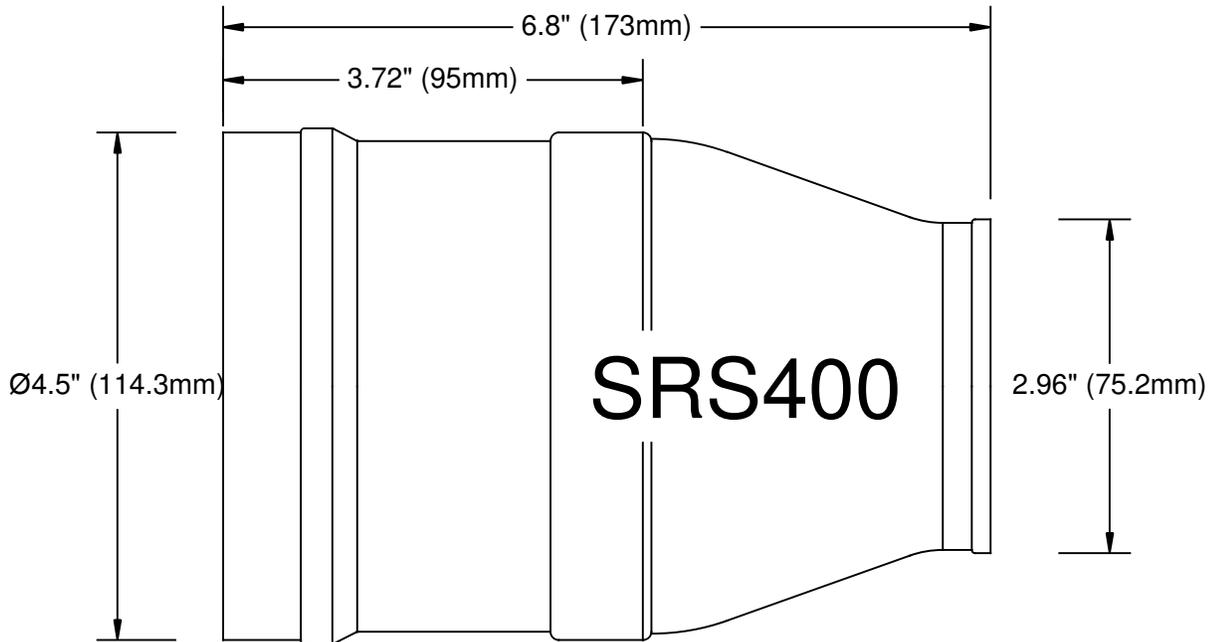
The Inlet Funnel is marked on back face of the flange for hole location if needed.
